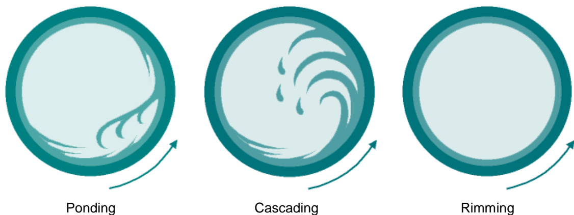
Figure 1: Condensate Behavior in a Dryer
